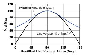
Figure 10. Switching Frequency vs. Phase Angle
