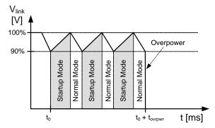
Figure 18. Overpower Protection Mechanism
