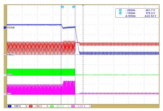
Figure 27. Overload — 240 mA to 500 mA, 90 VAC
