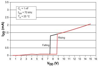
Figure 1. Supply Current vs. Supply Voltage
