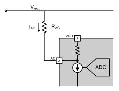
Figure 16. IAC Input Pin Model
