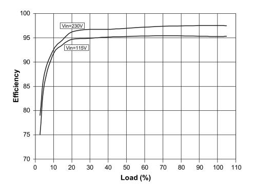
Figure 22. Efficiency vs. Load, Typical
