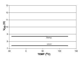
Figure 2. Start-up & UVLO vs. Temp
