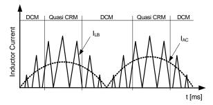
Figure 12. DCM and quasi-CRM Operation with CS1500
