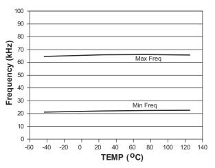
Figure 6. Min/Max Operating Frequency vs. Temp
