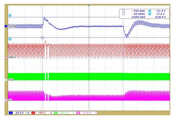
Figure 25. Load Transient — 20% to 80% (60 mA to 240 mA), 0.8 A/µsec Slew, 90 VAC
