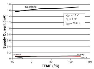
Figure 5. Supply Current ( $I_{SB}$ ,  $I_{ST}$ ,  $I_{DD}$ ) vs. Temp
