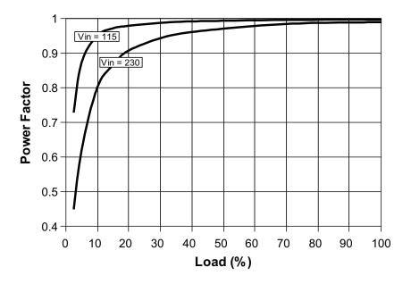
Figure 24. Power Factor vs. Load, Typical
