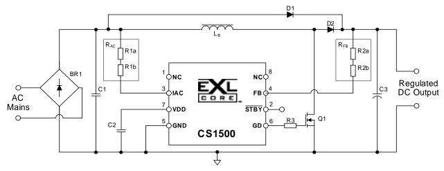
Figure 21. CS1500 Basic Application Circuit
