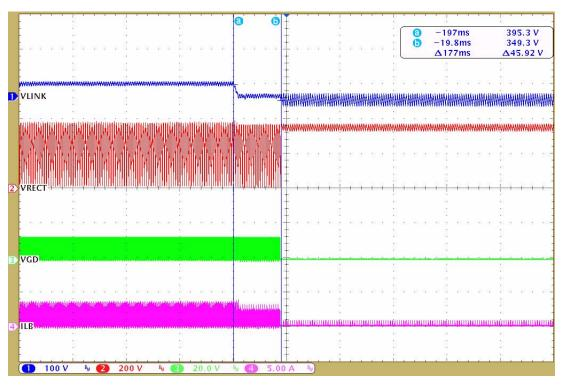
Figure 28. Overload — 240 mA to 500 mA, 265 VAC
