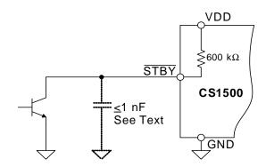
Figure 20. STBY Pin Connection
