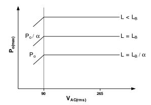
Figure 19. Maximal Output Power vs. Line Voltage
