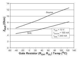
Figure 7. Gate Resistance ( $R_{OH}$ ,  $R_{OL}$ ) vs. Temp
