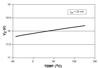
Figure 4. VDD Zener Voltage vs. Temp
