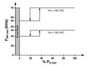
Figure 11. Switching Frequency vs. Output Power
