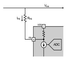
Figure 15. Feedback Input Pin Model
