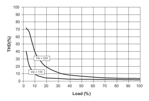
Figure 23. Distortion vs. Load, Typical
